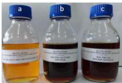
Figure 3.8. Samples of component additives: nano iron oxide nanoemulsion additive (a), water-in-oil nanoemulsion additive (b) and new generation nanoemulsion additives (c)
